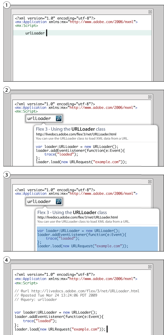
Figure 2. Example-centric programming with Blueprint. The user presses a hotkey to initiate a search; a search box appears at the cursor location (1). Searches are performed interactively as the user types; example code and running examples (when present) are shown immediately (2). The user browses examples with the keyboard or mouse, and presses Enter to paste an example into her project (3). Blueprint automatically adds a comment containing metadata that links the example to its source (4).
